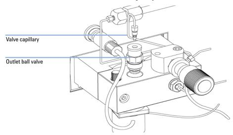
Figure 19 Exchanging the Outlet Ball Valve
