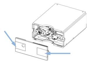
Figure 11 Removing the Front Cover
