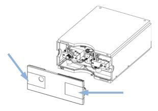
Figure 9 Removing the Front Cover
