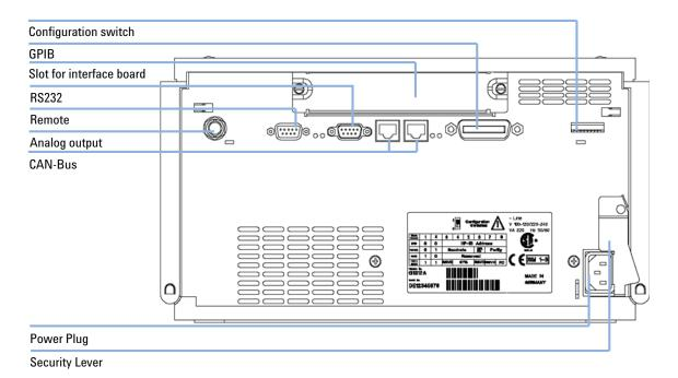
Figure 4 Rear View of Binary Pump - Electrical Connections and Label
