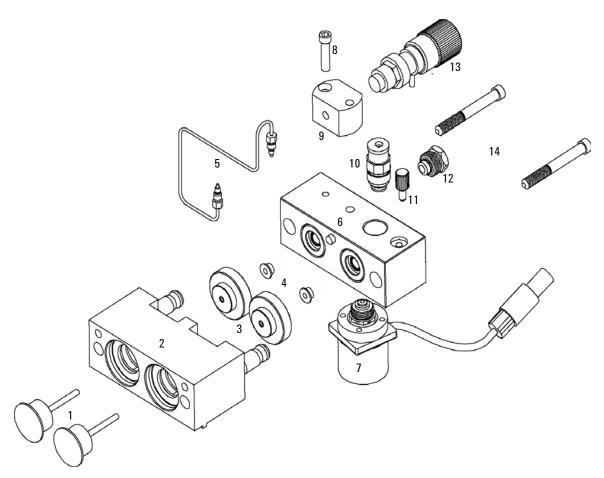
Figure 30 Pump-Head Assembly
