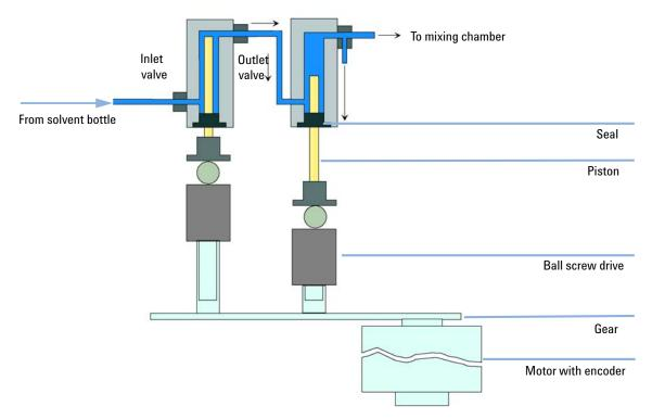
Figure 3 Principle of Pump Unit
