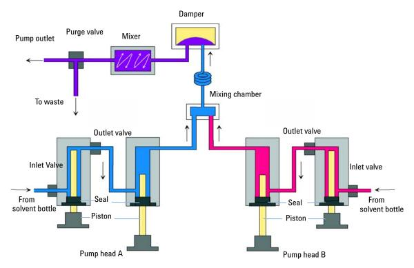
Figure 2 The Hydraulic Path
