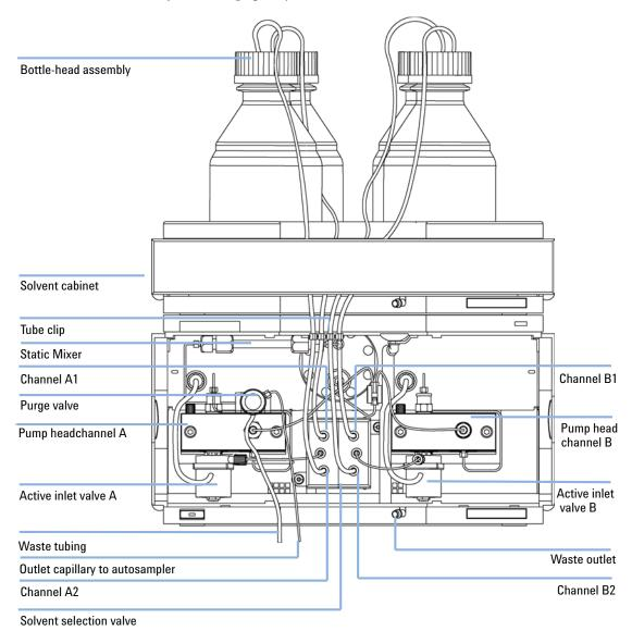
Figure 10 Binary Pump with Solvent Selection Valve
