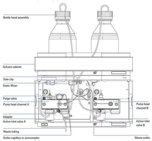
Figure 12 Flow Connection of Binary Pump Without Solvent Selection Valve
