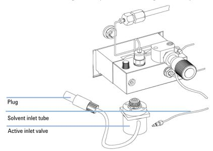
Figure 16 Exchanging the Active Inlet Valve
