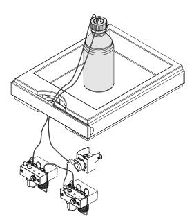
Figure 26 Pumphead after completed installation.
