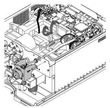
Figure 24 Wire connected to the mainboard.
