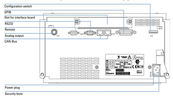
Figure 8 Rear of Binary Pump
