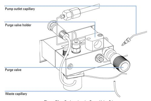
Figure 21 Exchanging the Purge Valve Frit
