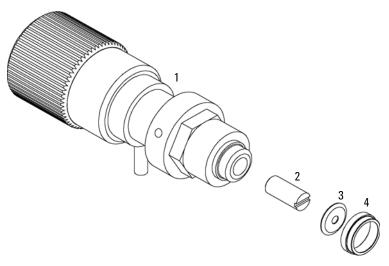
Figure 33 Purge-Valve Assembly
