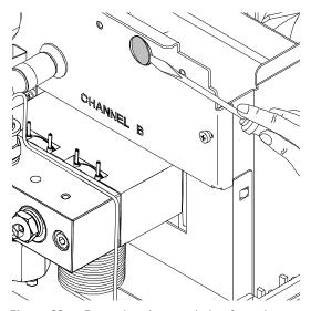
Figure 23 Removing the metal plug from the z-panel
