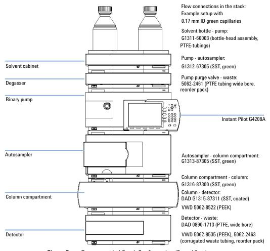
Figure 5 Recommended Stack Configuration (Front View)
