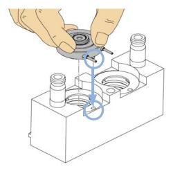
Figure 25 Inserting the active seal wash support rings.
