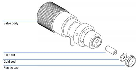
Figure 20 Purge Valve Parts
