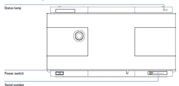
Figure 7 Front of Binary Pump
