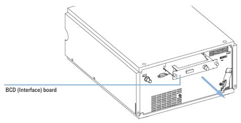
Figure 27 Exchanging the Interface Board
