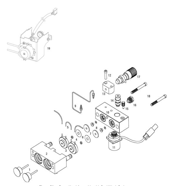
Figure 31 Pump Head Assembly with Seal Wash Option
