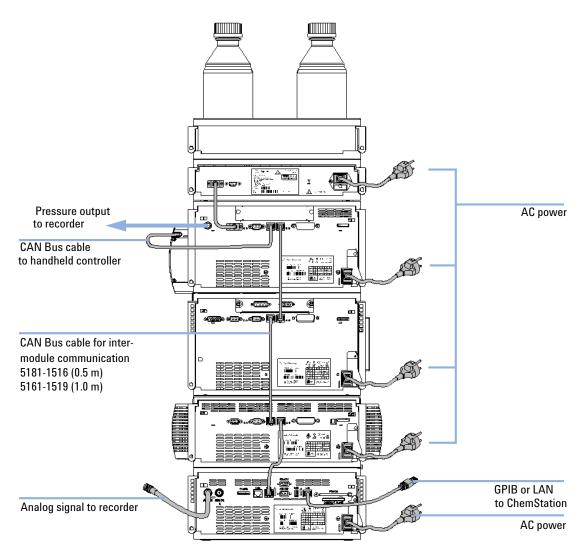
Figure 6 Recommended Stack Configuration (Rear View)
