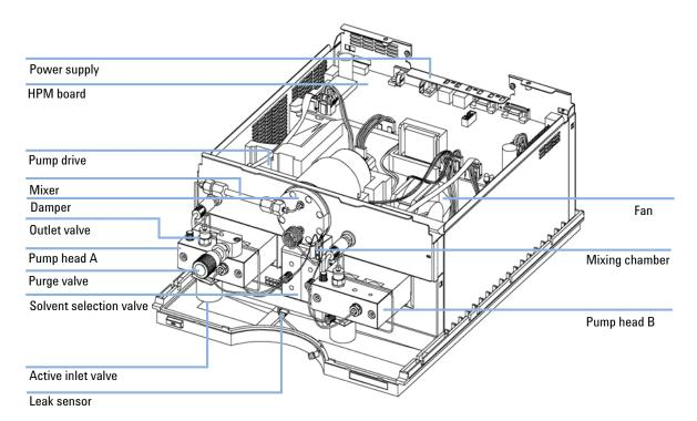
Figure 1 Overview of the Binary Pump
