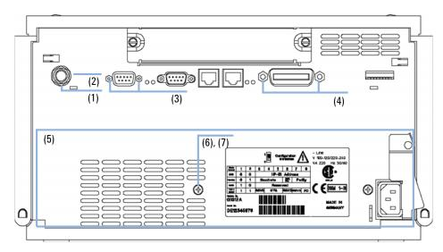
Figure 29 Overview of Main Assemblies (Rear View)
