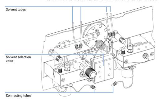
Figure 22 Exchanging the solvent selection valve
