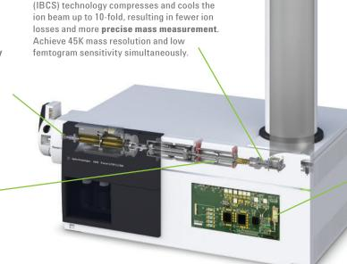
Agilent Ion Beam Compression and Shaping
