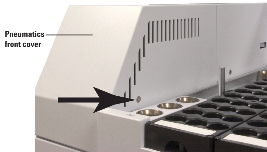
Figure 1 Remove the T-20 Torx screw from the pneumatics front cover
