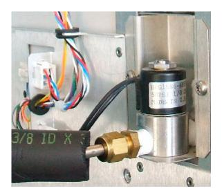
Figure 14 N<sub>2</sub> cryogenic cooling valve connections
