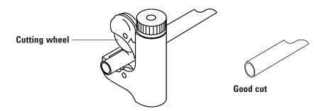
Figure 5 Typical tubing cutter
