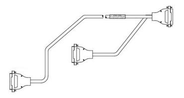
Figure 27 Remote start/stop cable, GC to Agilent instrument
