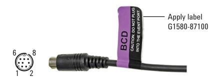
The BCD cable connector has eight passive inputs that sense total binary-coded decimal levels. The pin assignments for this connector are listed in Table 12.
