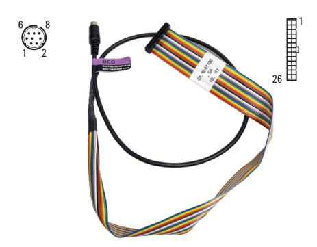
The BCD cable connector has eight passive inputs that sense total binary-coded decimal levels. The pin assignments for this connector are listed in Table 12.
