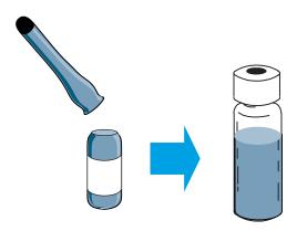
**2** Use a pipette to transfer the sample to a 2-mL screw-top vial. (If using an ALS, use a vial suitable for the ALS turret or tray.)
