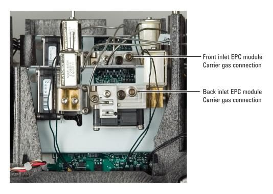
Figure 8 Inlet flow module
