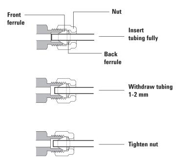
Figure 19 Insert the tubing
