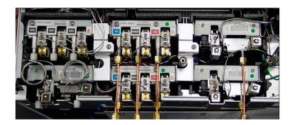
Figure 7 Plumbing flow modules
