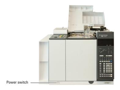
Figure 4 Power switch location
