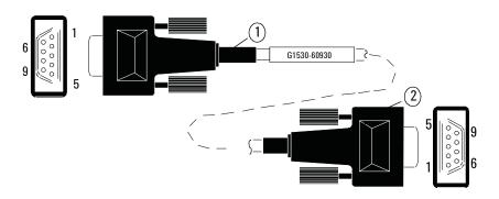
Figure 26 Remote start/stop cable, GC to Agilent instrument
