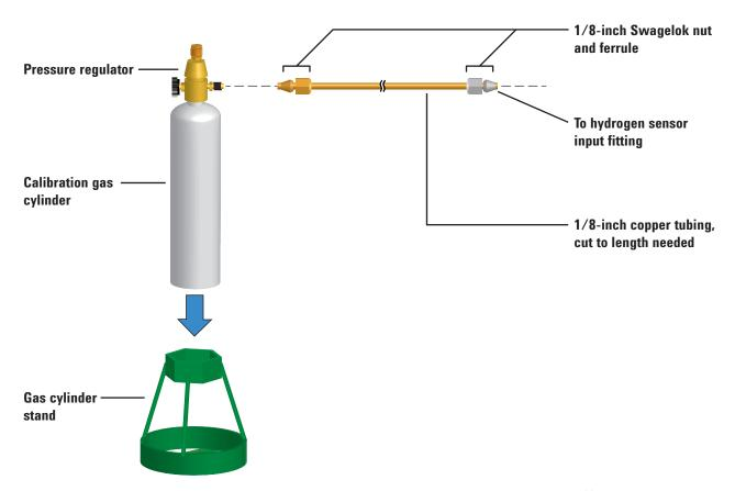
**2** Turn the pressure regulator completely off and set the output pressure as low as possible (full CCW).
