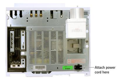
**3** Turn on the GC. The self-test diagnostic tests run automatically. If the screen displays **Power on successful**, continue with the installation procedure.
