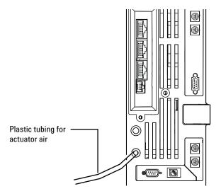
Figure 15 Valve actuator air tubing
