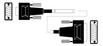
Figure 25 Remote start/stop cable, GC to Agilent integrator
