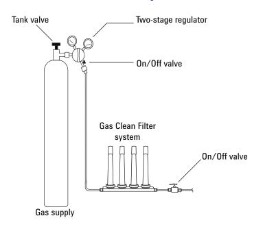
Figure 6 Plumbing the gas supplies
