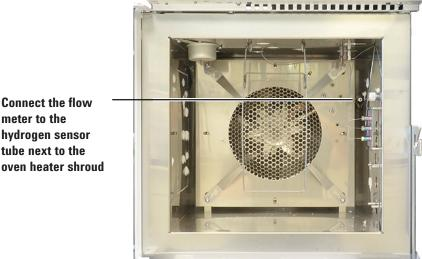
meter to the hydrogen sensor tube next to the oven heater shroud
