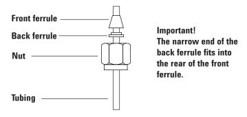
Figure 17 Swagelok nuts and ferrules
