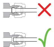
Figure 22 Completed fitting
