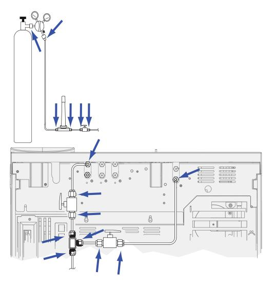
Figure 12 Locations to check for leaks
