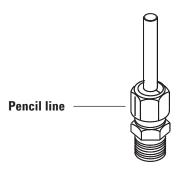
Figure 20 Marking the fitting
