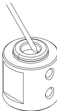
**16** The quartz body and the cell seal assembly can be separated for cleaning purpose.
