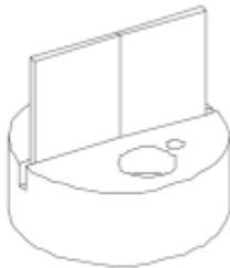
**4** Observe the orientation of the filter assembly top part. Install the assembly and fix the screws.
