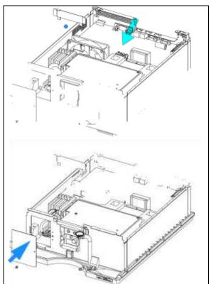
4 Replace the bumpers in the top foam so that they are positioned on the optical unit as shown.
