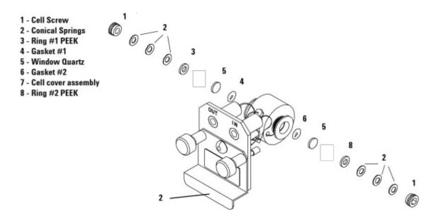
Figure 28 Standard Flow Cell (G1314-60086)
