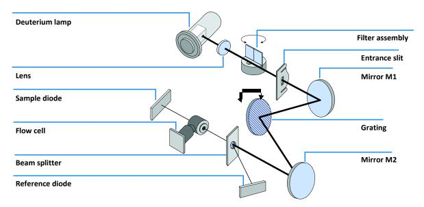
Figure 41 Optical Path of the Variable Wavelength Detector
