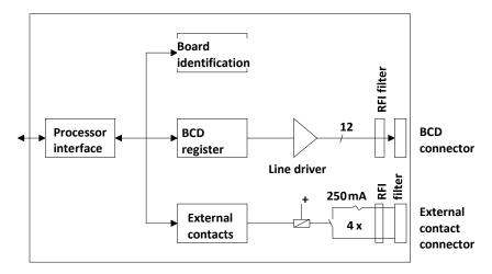
Figure 50 Block Diagram BCD Board LAN Board
