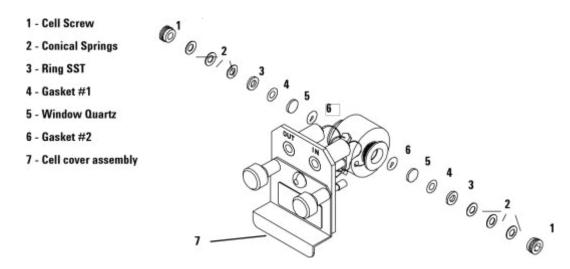
Figure 29 Standard Flow Cell
