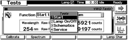
Use the F6 key (**Plot**) to view the signal. A simulated chromatogram (4 peaks) will repeat until the run is stopped. The signal is also available on the analog output. A change of the peakwidth will change the retention times.
