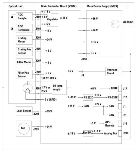
Figure 47 Power Interconnection Diagram of the Detector
