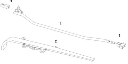
Figure 39 Power and Status Light Pipes
