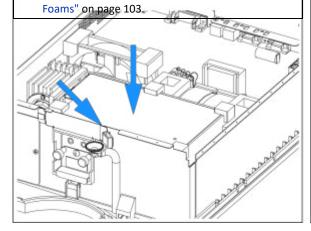
6 Observe the orientation of the filter assembly top part. Install the assembly and fix the screws.
