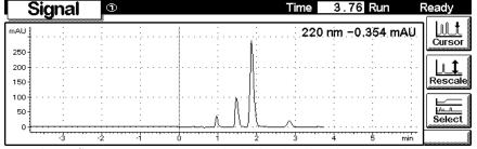
Press F6 key (**Select**). Here you can add additional online signals (maximum are 3), press F6 key (**Select**). Additional signals could be also pressure or temperature signals from other modules. Use the Right/Left arrows to switch between Available and
