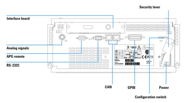
Figure 4 Rear View of Detector
