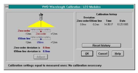
Figure 8 Wavelength Calibration
