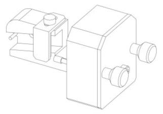
Figure 20 Cuvette Holder
