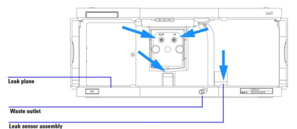
Figure 21 Drying the Leak Sensor
