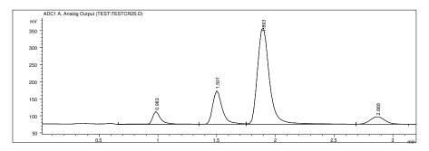
Figure 14 Test Chromatogram on Integrator (response time 2 seconds)
