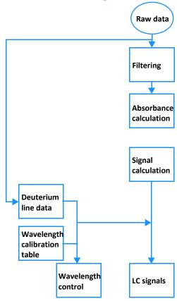
Figure 49 Firmware Flow Diagram
