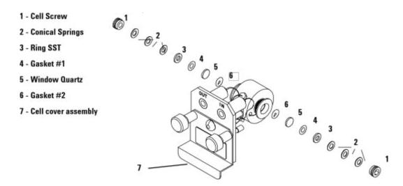
Figure 31 Micro Flow Cell
