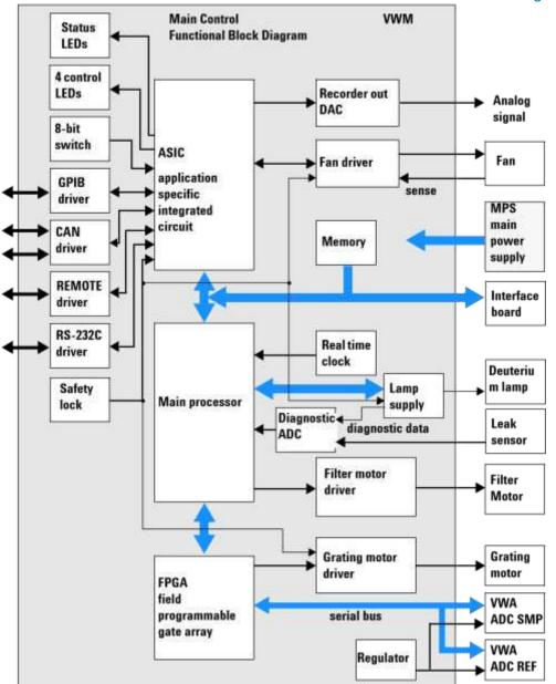
Figure 46 Block Diagram VWD Main Controller Functionality
