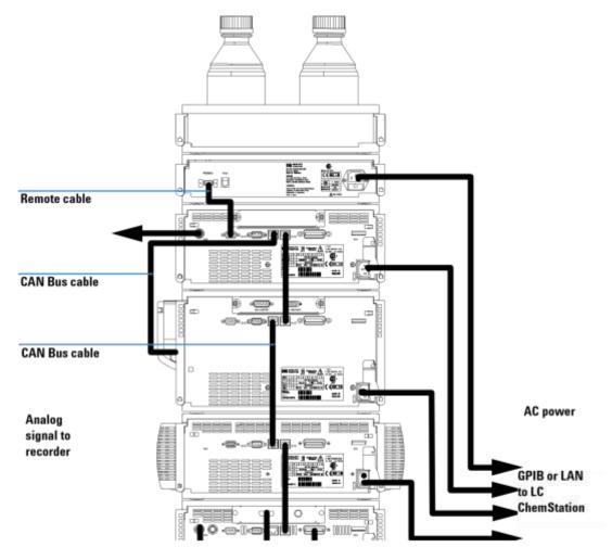
Figure 2 Recommended Stack Configuration (Rear View)
