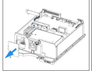
**3** Disconnect the deuterium lamp connector and all cables coming from the optical unit to the main board.
