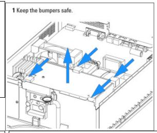
2 Remove the lamp cover and the plate above the flow
