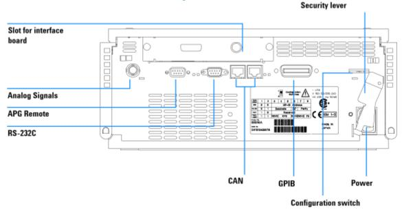
Figure 45 Electrical Connections
