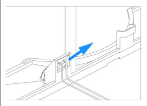
8 Replace the leak sensor assembly into the leak panel and route the cable through the cabinet and foam channel. Reconnect it to the main board.
