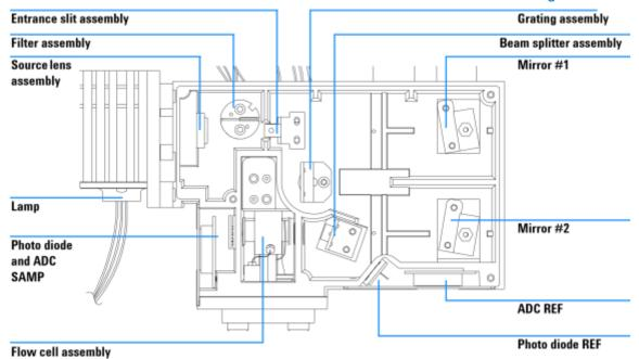
Figure 42 Mechanical Layout of the Optical Unit
