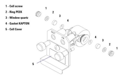
Figure 33 High Pressure Flow Cell
