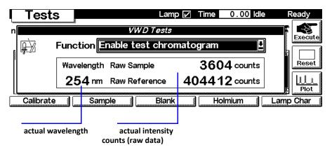
Figure 9 Photocurrent Readings on Control Module
