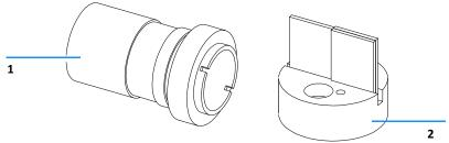
Figure 27 Source Lens and Filter Assembly Standard Flow Cell (G1314-60086)
