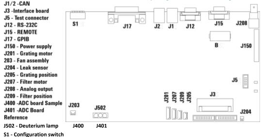
Figure 24 Location of Connectors on VWM Board
