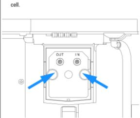
3 Unscrew the thumb screws parallel and remove the flow
