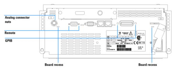
Figure 23 Unscrew Connectors From Board
