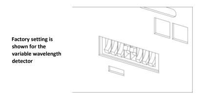
Figure 52 8- bit Configuration Switch
