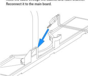
9 Replace the leak base by pressing it into the bottom of the cabinet.
