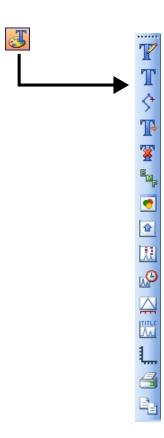
$\begin{array}{ll} \textbf{Integration Tool Set} & \textbf{Allows you to perform integration and reporting tasks on a chromatogram.} \end{array}$
