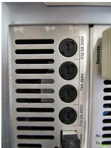
Figure 67 AC Board fuses
