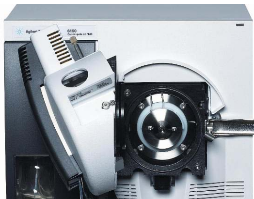
Figure 14 Opened electro spray Agilent Jet Stream Technology spray chamber
