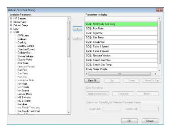
c Add all the parameter values you intend to monitor, and click the **OK** button. Parameters that you may want to monitor include MS values (such as heater, and vacuum pressure) or LC values (such as binary pump, column, DAD, etc.) You can set the background and text color for each parameter. You can also set a range for the parameters which are numbers. If the value of the parameter is not within the limits which you entered, then the background of the parameter is set to red.
