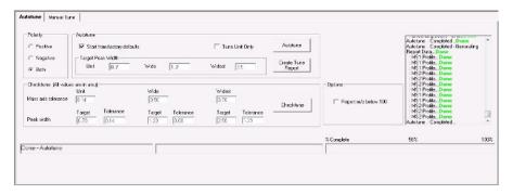
2 Click **Checktune** to evaluate if the MS parameters are within the limits to produce the specified mass accuracy and resolution. Checktune takes approximately 3 minutes to run for each polarity.
