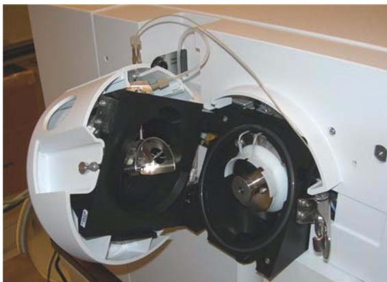
**Figure 1** Opened electrospray spray chamber
