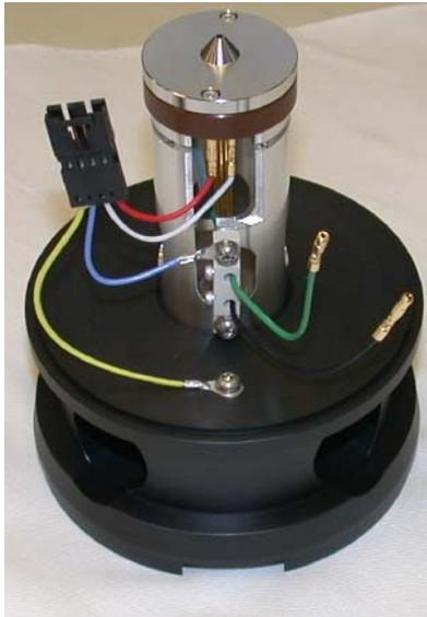
**Figure 52** Ion optics assembly
