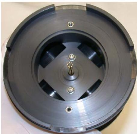
**Figure 54** Octopole rods extending through Skimmer Spacer.
