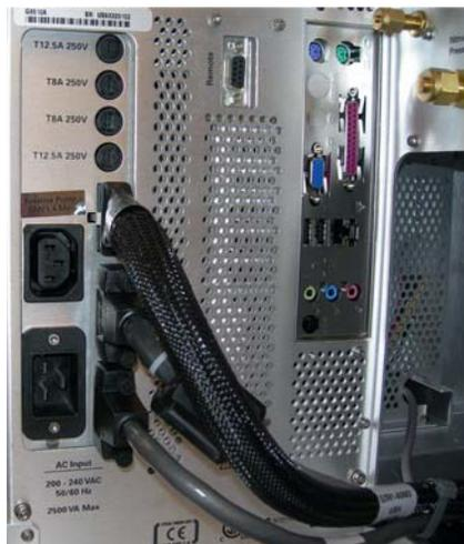
**Figure 64** Disconnect the instrument power cable.
