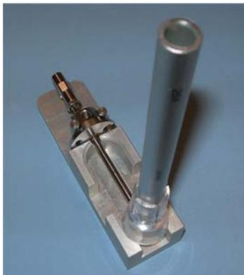
**Figure 36** Electrospray nebulizer needle in needle holder
