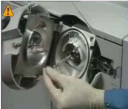
**Figure 45** Reinstalling the capillary
