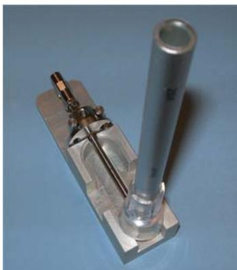
**Figure 6** Electrospray nebulizer needle in needle holder
