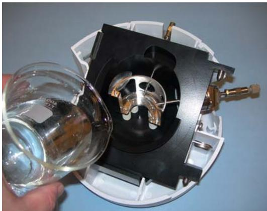
**Figure 2** Filling the spray chamber
