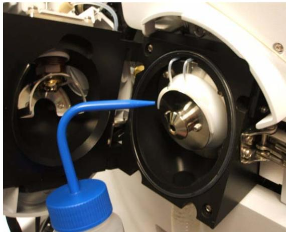
**Figure 4** Rinsing the area around the spray shield
