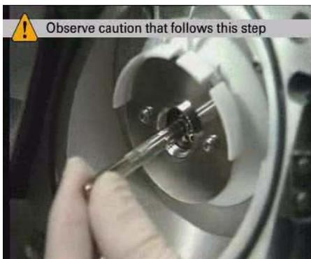
**Figure 44** Pulling the capillary out of the desolvation assembly
