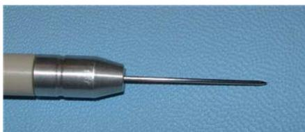
**Figure 33** APCI corona needle after cleaning.
