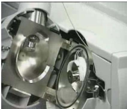
**Figure 24** Opened spray chamber
