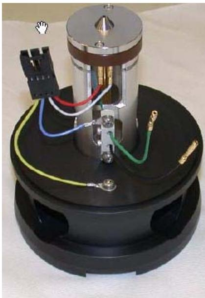
**Figure 61** The re-assembled ion optics assembly
