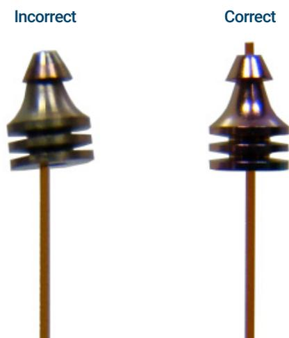
Figure 18. Incorrect and correct swaging symmetry
