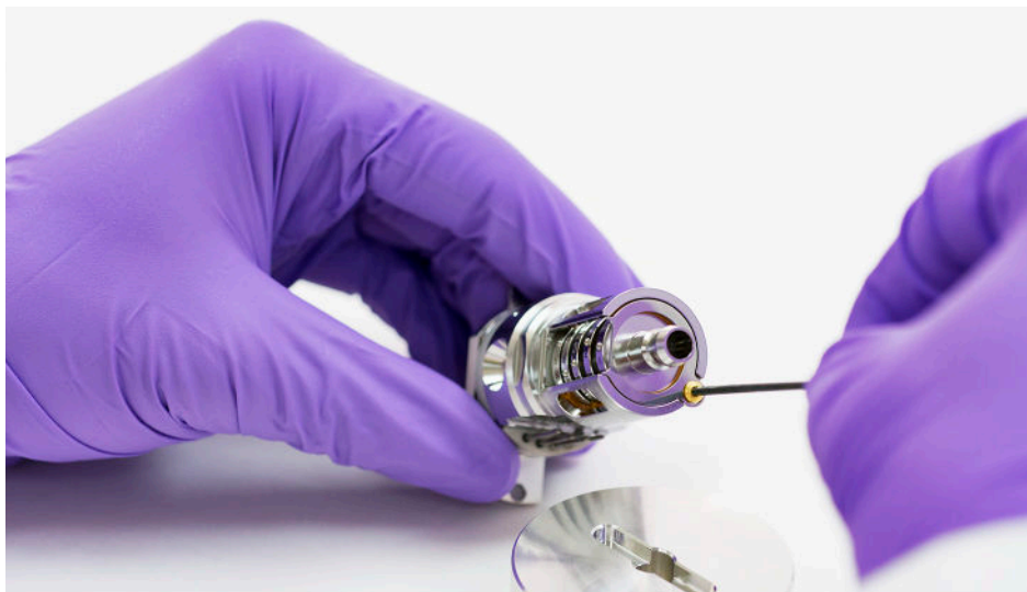
Figure 57. Secure the lens screw and locking ring insulator
