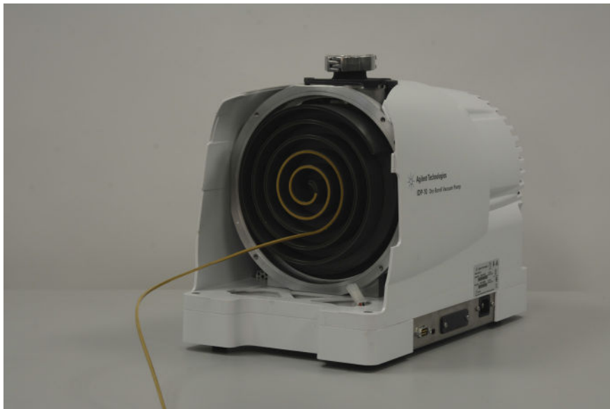
Figure 18. Installing a new tip seal
