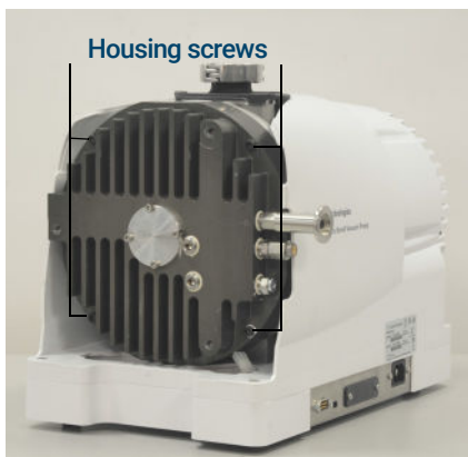
Figure 16. Removing the scroll housing
