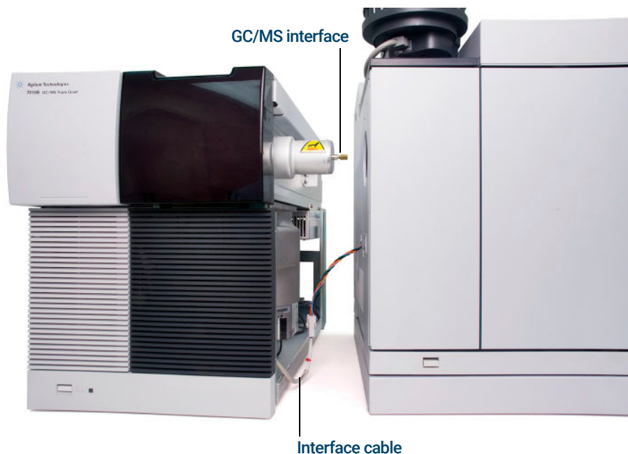
Figure 5. Separating/connecting the MS and GC
