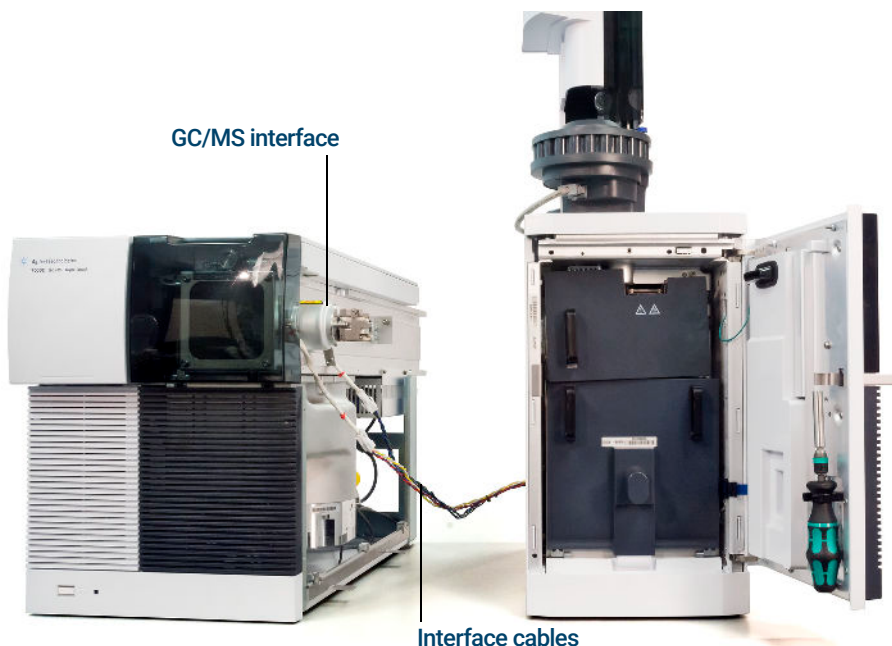
Figure 6. Separating/connecting the MS and 9000 GC
