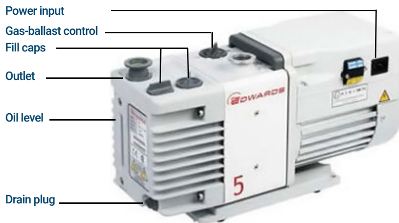
Figure 12. Rotary vane foreline pump
