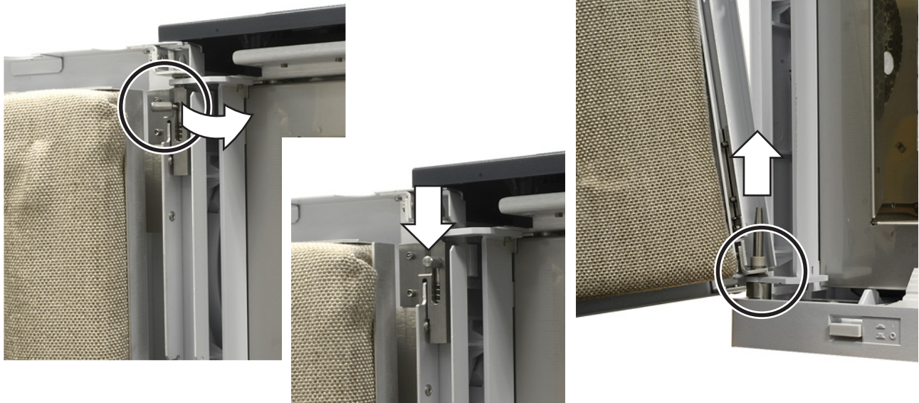
Figure 2 Removing the oven door
