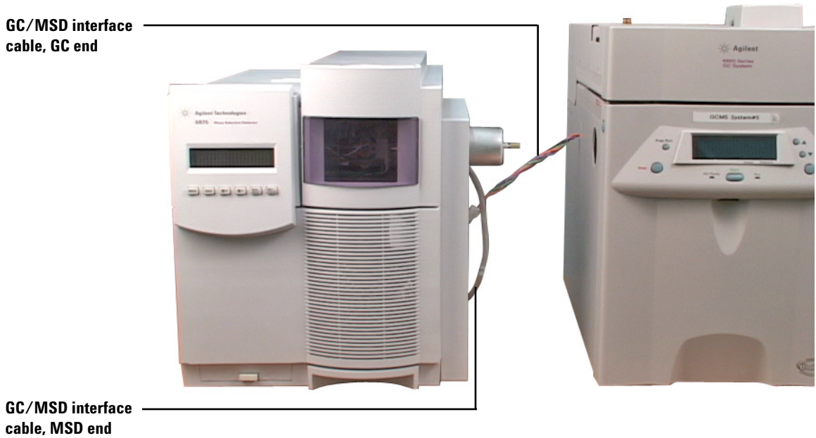
Figure 11 Interstitial panel installed, GC/MSD interface cable connected
