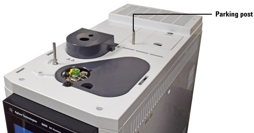
Figure 10 Installing the parking post on an Intuvo 9000 GC
