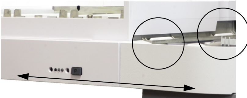
Figure 5 Sample tray correctly installed.
