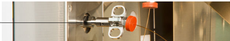
Figure 61 GC/MSD interface with a self tightening column nut
