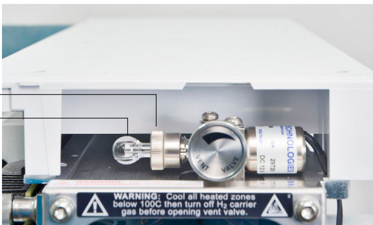
Figure 15 Removing the EI calibration vial
