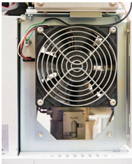
Figure 30 Diffusion pump with fan
