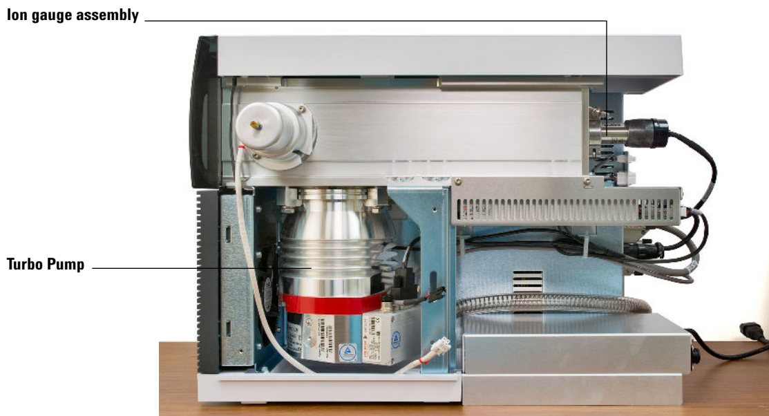
Figure 53 Turbo pump and related parts
