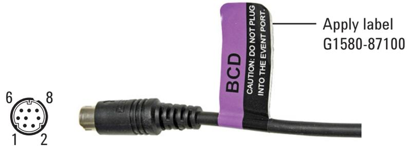
The BCD cable connector has eight passive inputs that sense total binary-coded decimal levels. The pin assignments for this connector are listed in [Table 12](#).
