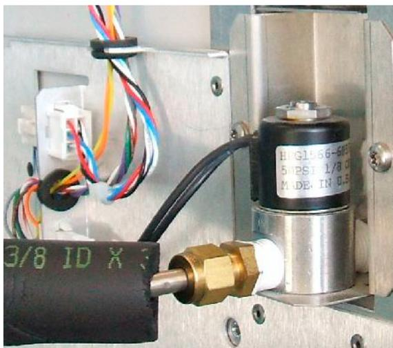
**Figure 14** N<sub>2</sub> cryogenic cooling valve connections
