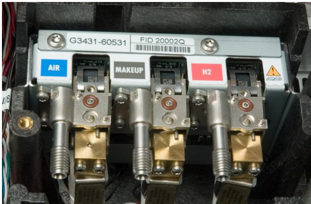
**Figure 10** Detector flow module
