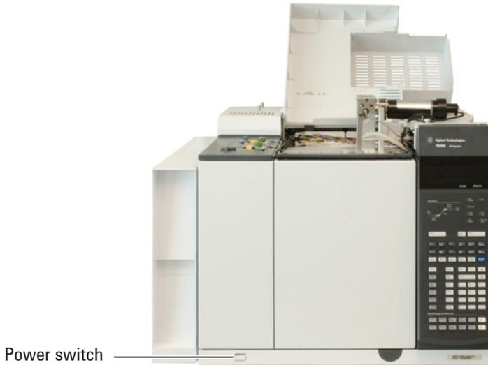
**Figure 4** Power switch location
