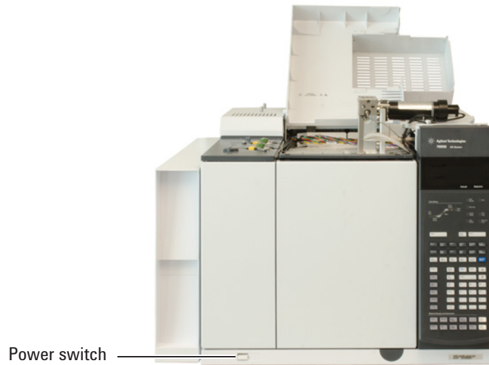
Figure 4 Power switch location
