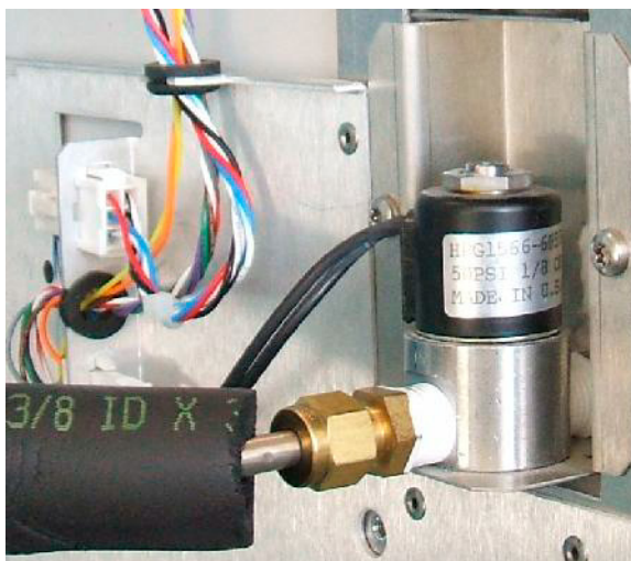
Figure 14 N 2 cryogenic cooling valve connections
