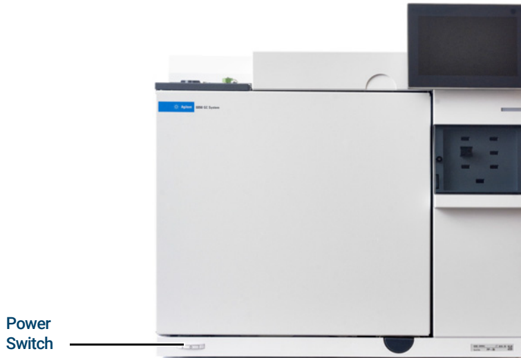
Figure 6. Power switch location
