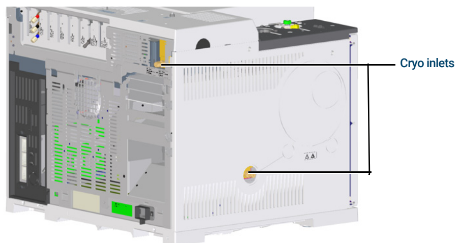
Figure 13. Location of cryogenic cooling valve
