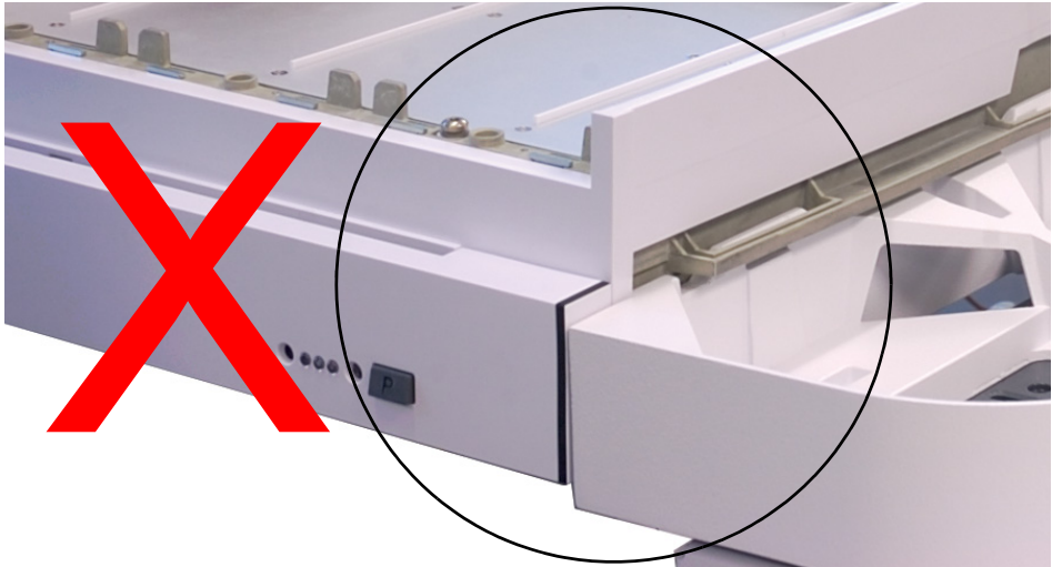
Figure 6 Sample tray incorrectly installed.
