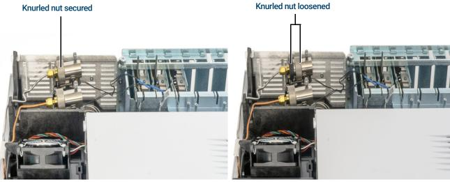
Figure 38. Loosen knurled nut
