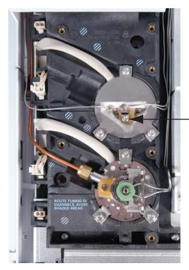
7 Lift the interface out of the heater block.
