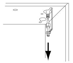
5 Unscrew and remove the adapter cap.
