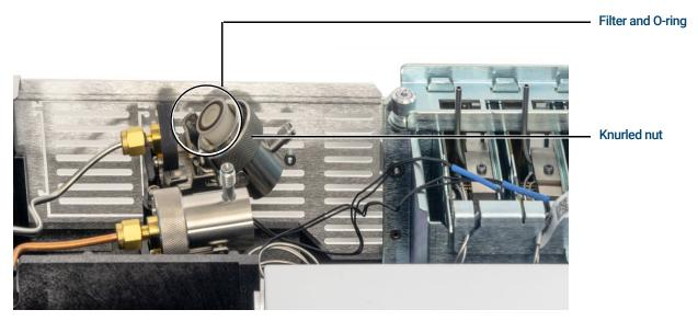
Figure 31. Slide trap assembly to expose the filter
