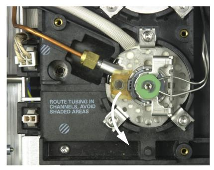
4 Loosen the O-ring from the sealing surface with tweezers.
