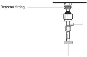
11 Tighten the nut finger-tight and then use a 9/16-inch wrench to tighten until snug.
