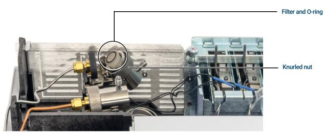
Figure 39. Slide trap assembly to expose the filter
