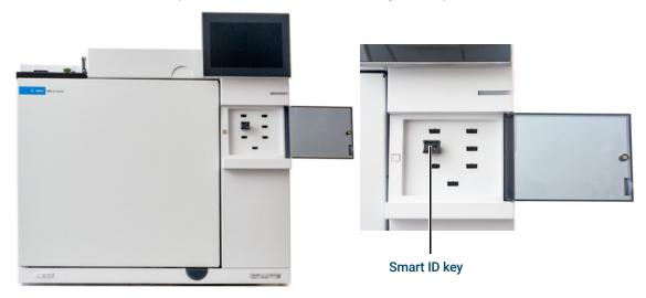
Figure 21. Insert Smart ID key
