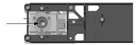
17 Pull the jet straight out of the detector. Use tweezers, if necessary.
