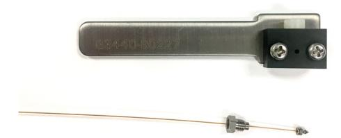
Figure 7. Thread the column through the internal nut, ferrule, and swaging tool
