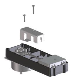
**9** Remove the screws that secure the electrometer, then lift up and set aside.
