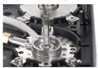
6 Inspect the surface of the gold seal for graphite or rubber septum contamination. If required, replace the gold seal. See "To Replace the Gold Seal on the Split/Splitless Inlet" on page 65.
