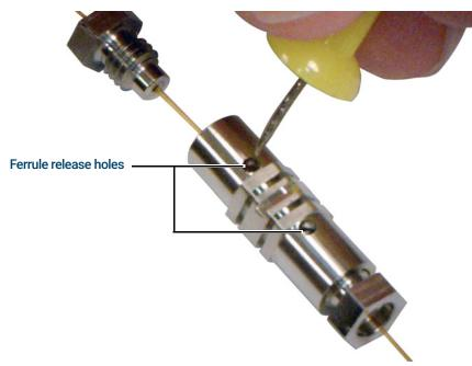
Figure 19. Release the ferrule (Ultimate Union fitting shown)
