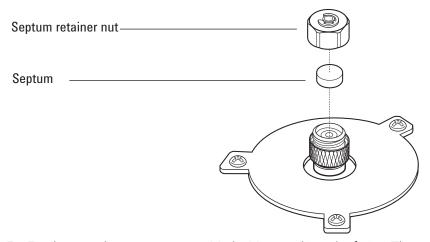
**5** Firmly press the new septum or Merlin Microseal into the fitting. The metal parts side of the Merlin Microseal should face down (toward the oven).
