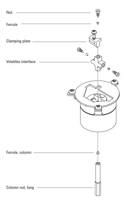
Figure 36. Volatiles interface exploded parts
