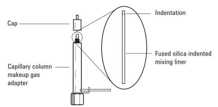
9 Place a new 1/4-inch Swagelok nut and ferrule onto the makeup gas adapter.
