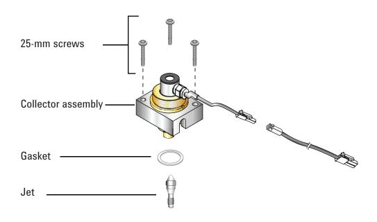
Figure 41. FID exploded parts view
