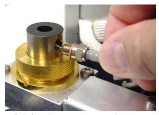
**b** Tighten the ignitor with a wrench. Ignition requires a good electrical contact that is free of any dirt.
