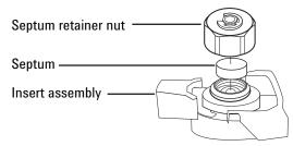
5 Firmly press the new septum or Merlin Microseal into the fitting. The metal parts side of the Merlin Microseal should face down (toward the oven).
