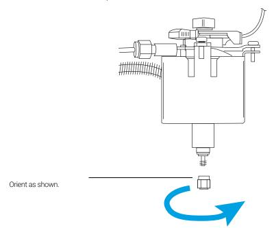
The nut must spin freely before it can be used to install a column.
