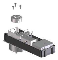
7 Remove the screws that secure the cover base, then lift up the cover base and set aside.
