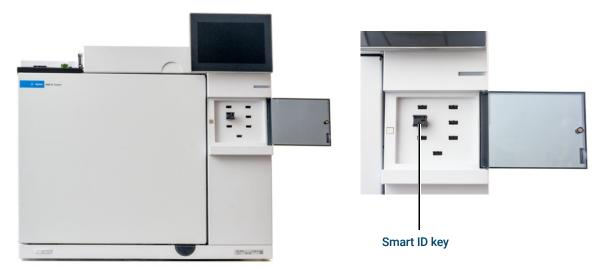
Figure 33. Insert Smart ID key
