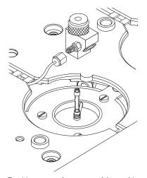
5 Unscrew the assembly tool into two pieces: the ferrule guide and the compression fitting.
