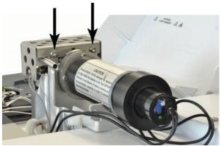
5 For a single wavelength FPD, remove the two screws at the bottom left of the cover.
