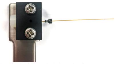
Figure 8. Thread the internal nut into the swaging tool
