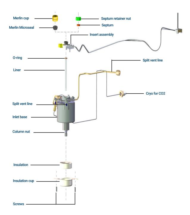
Figure 28. Multimode inlet exploded parts
