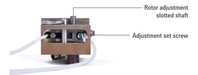
**b** Locate the rotor adjustment shaft on top of the actuator. Use a screwdriver to rotate the valve rotor counterclockwise until it stops.
