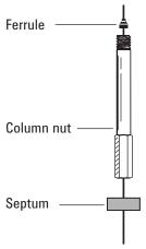
5 Score the column using a glass scribing tool. The score must be square to ensure a clean break.
