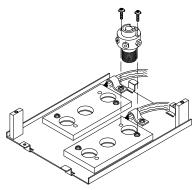
11 Use needle-nosed pliers to move the valve rotor index pin of the valve counterclockwise until the pin touches the valve stop **Off** position.
