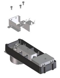
8 Remove the screws that secure the interconnect cover, then lift up the cover and set aside.
