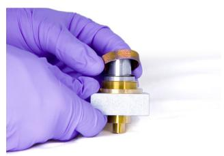
**c** Lift the castle out of the collector housing. When removing the castle, some of the collector parts may be attached. Set these on a clean cloth to protect from scratches or dirt.
