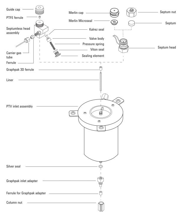
Figure 32. Programmable temperature vaporization inlet exploded parts
