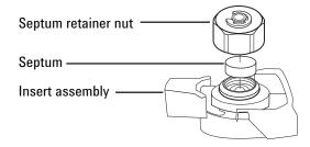
**5** Firmly press the new septum or Merlin Microseal into the fitting. The metal parts side of the Merlin Microseal should face down (toward the oven).
