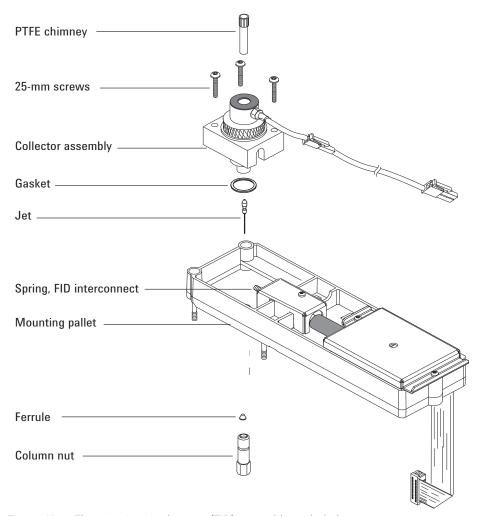
Figure 40. Flame ionization detector (FID) assembly exploded parts
