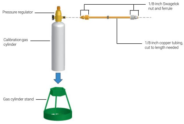
Figure 5. Hydrogen sensor calibration gas cylinder parts identification
