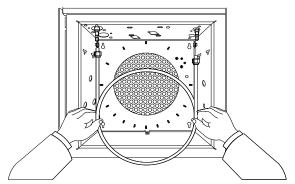
**8** Withdraw the column 1 to 2 mm from both the inlet and detector. Finger-tighten both column nuts.
