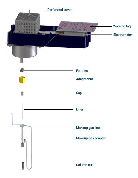
Figure 47. Electron Capture Detector (ECD) exploded parts
