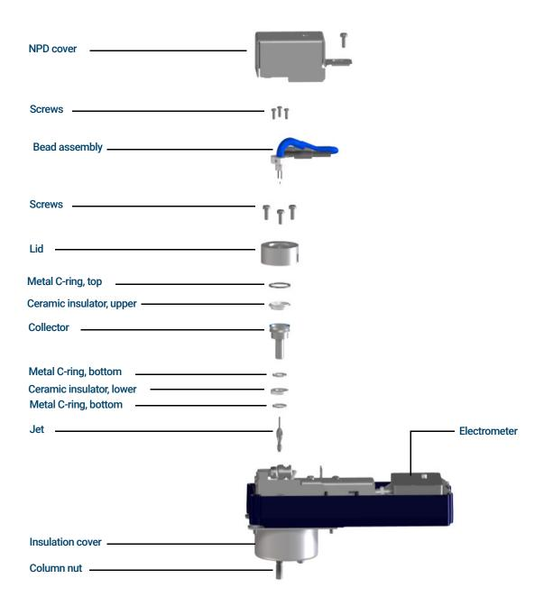
Figure 43. Nitrogen-Phosphorus Detector (NPD) exploded parts
