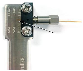
Figure 15. Align column (split/splitless shown)
