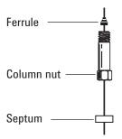
4 Score the column using a glass scribing tool. The score must be square to ensure a clean break.
