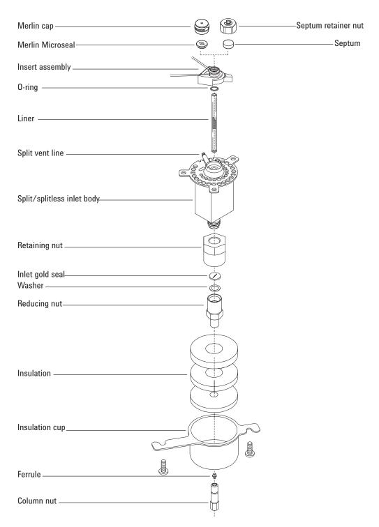
Figure 20. Split/splitless inlet exploded parts
