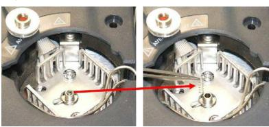
**6** Remove the existing insert from the inlet by gently pushing it out from below with a wire or piece of column. Store the insert for possible later use.
