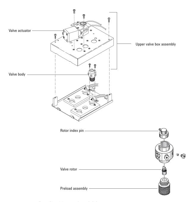
Figure 51. GC rotary valve exploded parts
