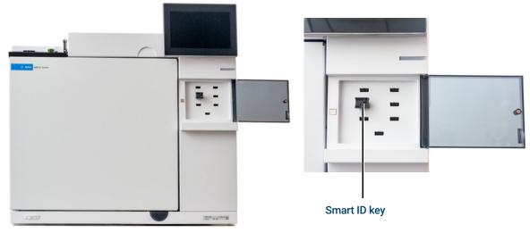
Figure 25. Insert Smart ID key
