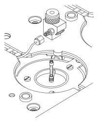
5 Unscrew the sealing element from the head assembly and carefully remove the Viton seal and the pressure spring
