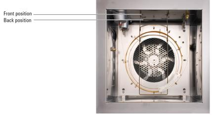
3 Insert the ends of the hanger into the slots in the selected position.
