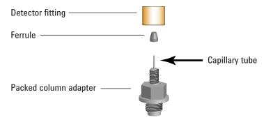
4 Carefully install the adapter assembly into the detector fitting. Align the adapter so the it enters the detector fitting as vertically as possible. Avoid stressing the adapter capillary tube. Finger-tighten the adapter into the detector base, then tighten an additional 1/8 turn using a wrench.
