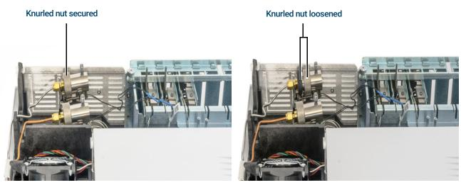
Figure 22. Loosen the knurled nut
