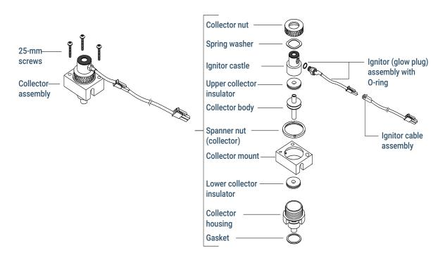
Figure 42. FID collector assembly exploded parts view
