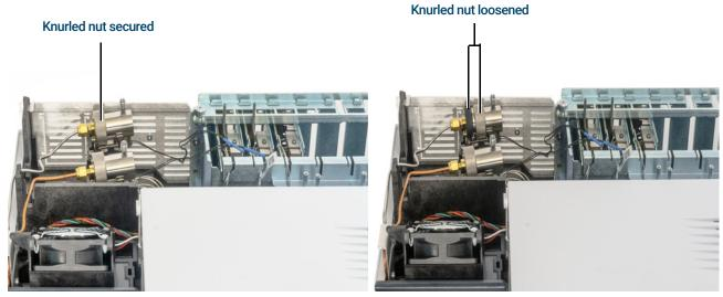
Figure 34. Loosen knurled nut
