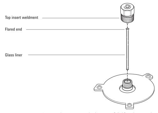
4 Use a thin wire or wood splint to carefully lift and remove the old glass liner.
