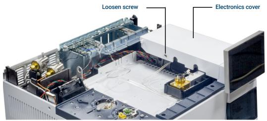
Figure 3. 8890 GC electronics cover
