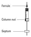
**6** Score the column using a glass scribing tool. The score must be square to ensure a clean break.
