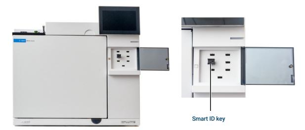
Figure 29. Insert Smart ID key
