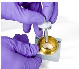
**b** Remove the lower insulator with tweezers and place the parts on a clean cloth.
