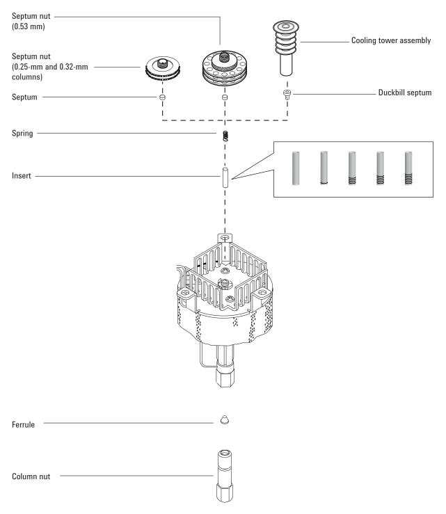
Figure 26. Cool on-column inlet exploded parts
