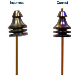
Figure 18. Incorrect and correct swaging symmetry
