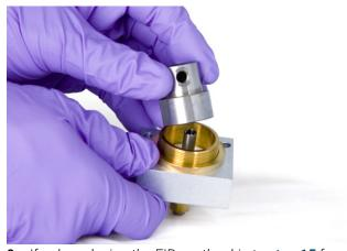
9 If only replacing the FID castle, skip to step 15 for reassembly.
