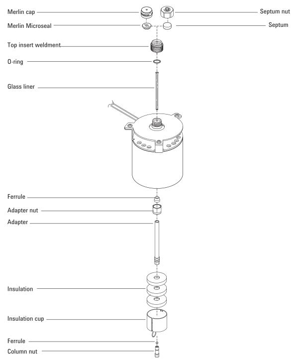
Figure 24. Purged packed inlet exploded parts
