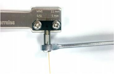
Figure 16. Tighten the column nut
