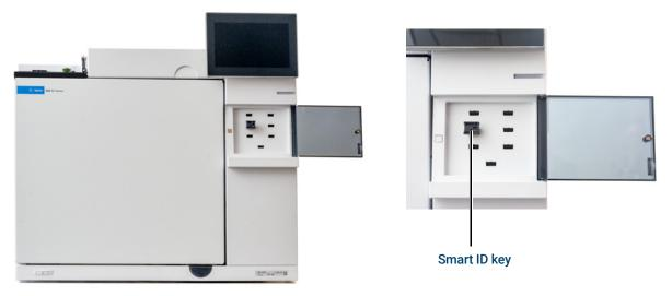
Figure 37. Insert Smart ID key
