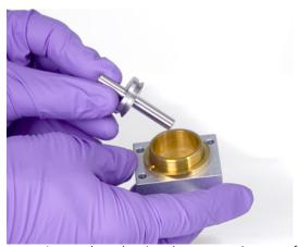
**c** Insert the other insulator onto the top of the collector, with the flat surface facing towards the housing.
