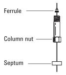
5 Score the column using a glass scribing tool. The score must be square to ensure a clean break.
