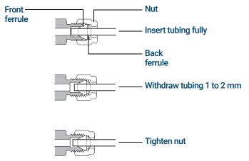
Figure 54. Insert the tubing
