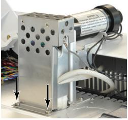
6 Lift the cover off the detector.
