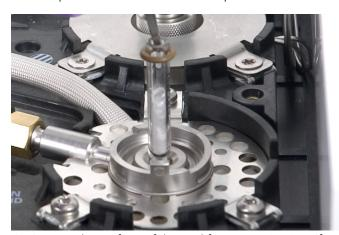
6 Inspect the surface of the seal for contamination. If required, clean with cotton swabs.
