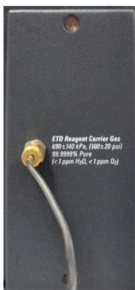
Figure 2-29. ETD reagent carrier gas port at the ETD Module
