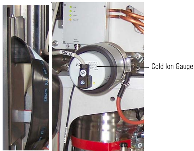
Figure 2-31. Electronic connections to linear trap
