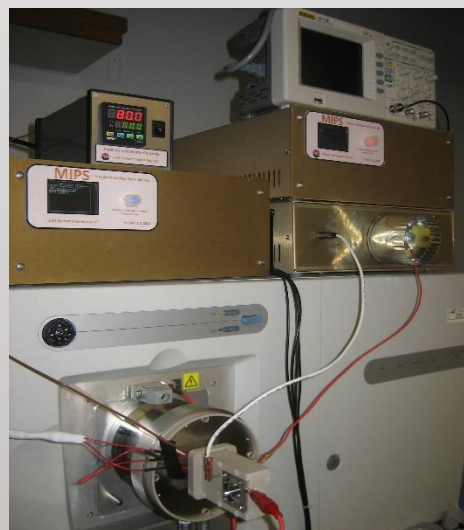
Complete FAIMS/LTQ XL system with ETD capability
