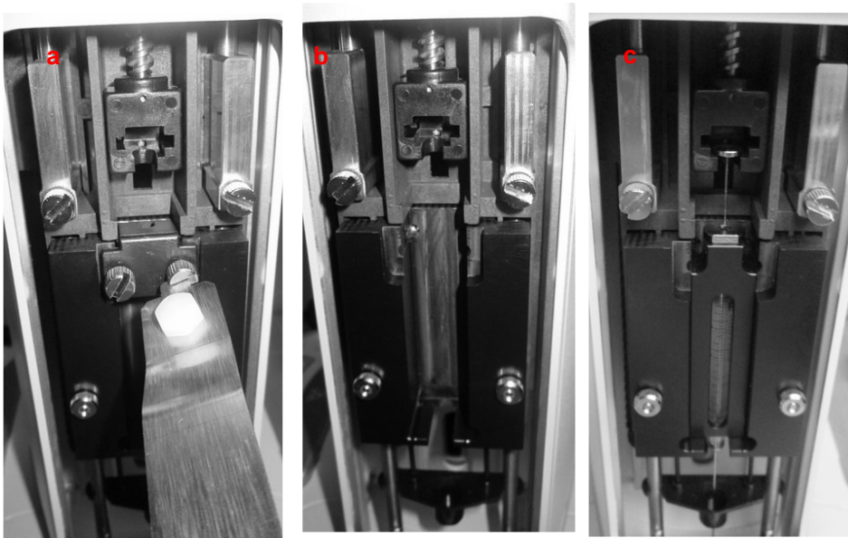
Figure 157: Liquid syringe installation
