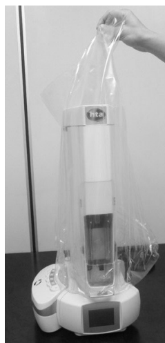
Figure 51: Remove the protection belt Figure 52: Remove the polythene bag
