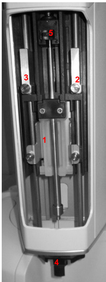
Figure 25: Fiber holder location (SPME mode)
