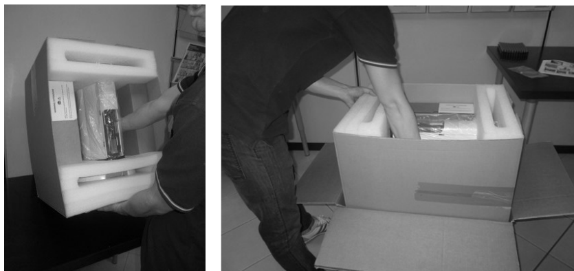
Figure 210: Put the autosampler in the box
