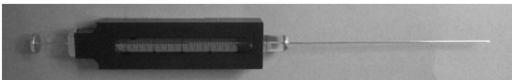
Figure 212: Syringe with syringID adapter containing the RFID tag
