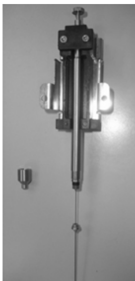
Figure 200: Fiber mounting in the Fiber holder_2
