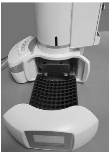
Figure 152: Rack for 2ml vials installation
