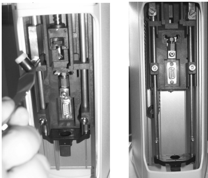
Figure 61: Moving from shipping to operating position Figure 62: Operating position
