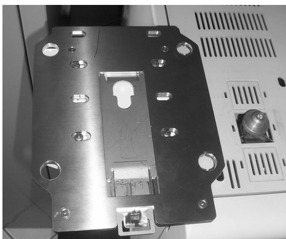
Figure 55: Example of a mounting plate correctly mounted on a GC
