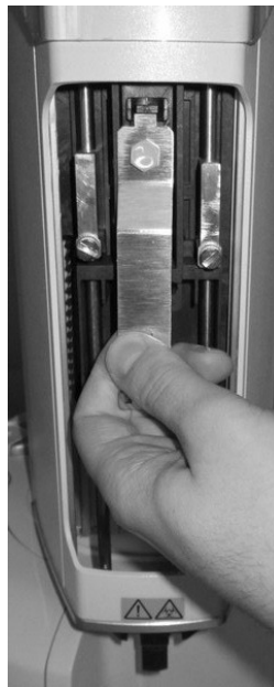
Figure 132: Plunger locker removing
