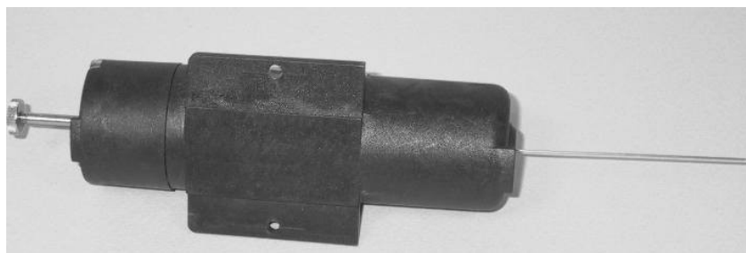
Figure 12: Syringe warmer assembly (Headspace mode)
