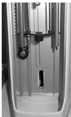
Figure 170: Change from liquid to Headspace mode_Remove vial locator
