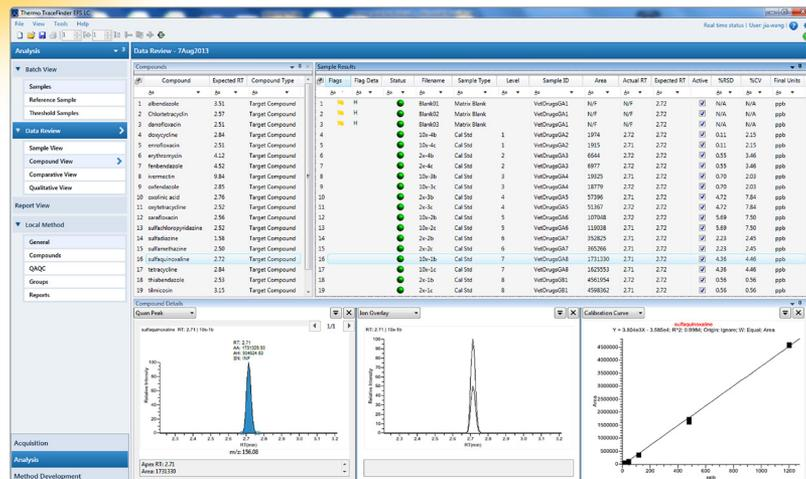
TSQ Endura MS provides sensitive, accurate quantitation of 21 antibiotics with results for sulfamonomethoxine from 0.48 ng/mL to 1200 ng/mL shown here
