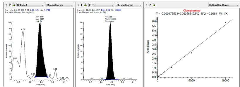
Analysis of clomipramine, a tricyclic antidepressant (TCA), in human plasma at LOQ of 1 ng/mL showing quantifying ion, internal standard ion, and calibration curve
