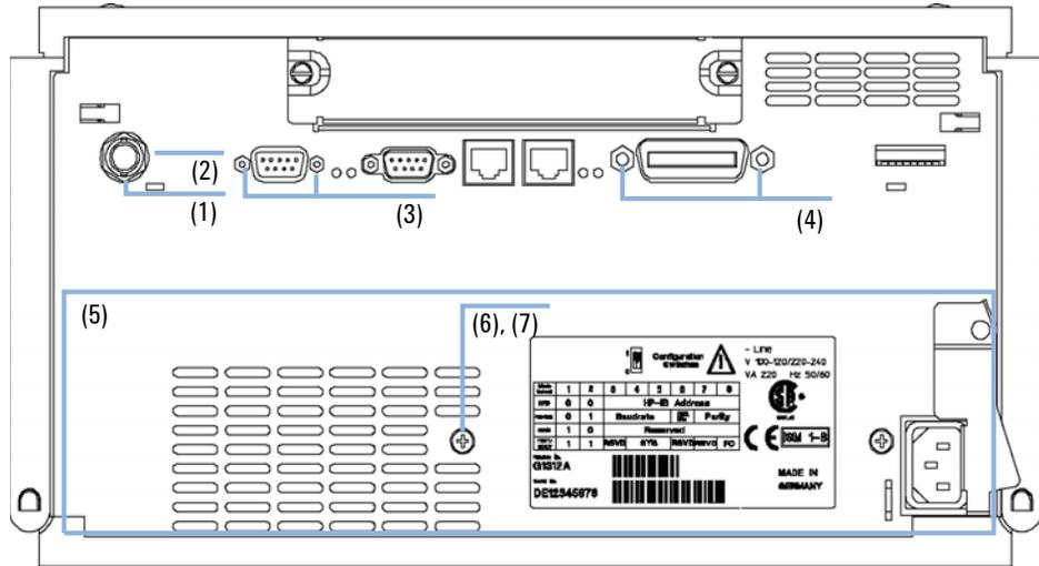
**Figure 29** Overview of Main Assemblies (Rear View)
