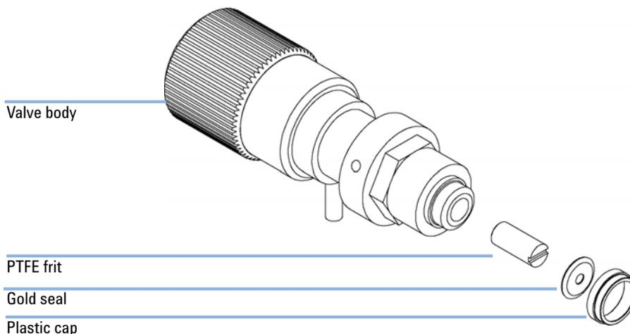
**Figure 20** Purge Valve Parts
