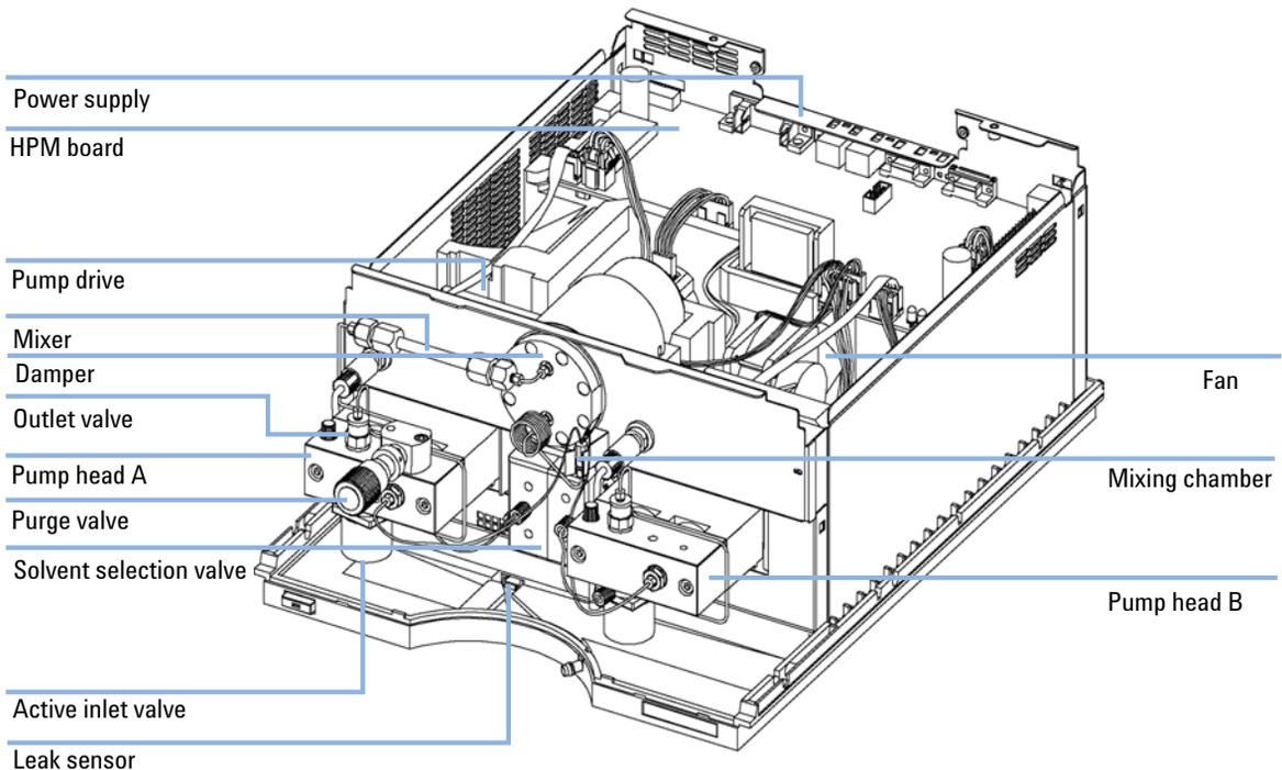
**Figure 1** Overview of the Binary Pump
