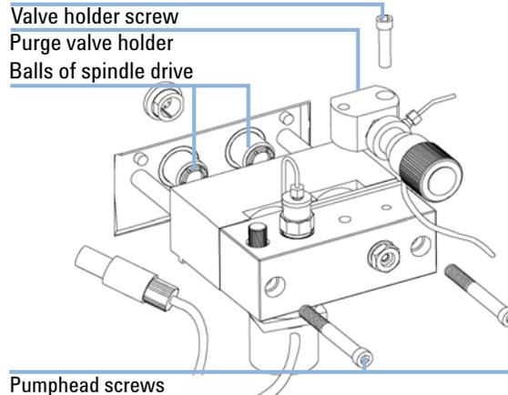
**2** Using a 4 mm hexagonal key tighten the pumphead screws stepwise with increasing torque.
