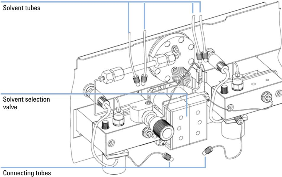
**Figure 22** Exchanging the solvent selection valve
