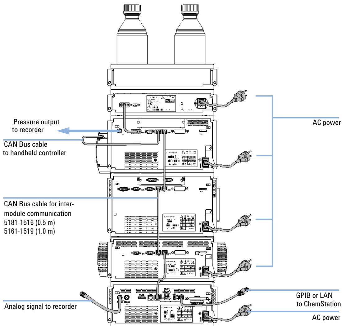
**Figure 6** Recommended Stack Configuration (Rear View)
