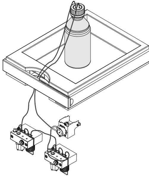
**Figure 26** Pumphead after completed installation.
