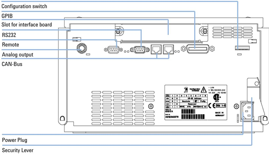
**Figure 4** Rear View of Binary Pump - Electrical Connections and Label
