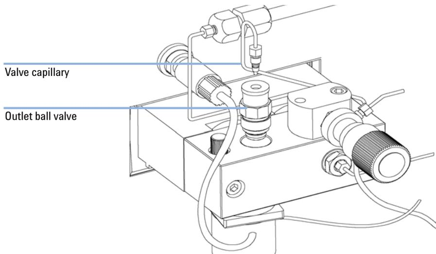
**Figure 19** Exchanging the Outlet Ball Valve
