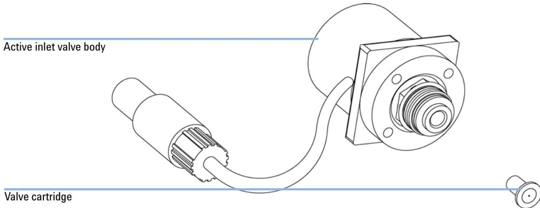
**Figure 17** Active Inlet Valve Parts
