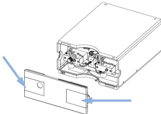
**Figure 11** Removing the Front Cover
