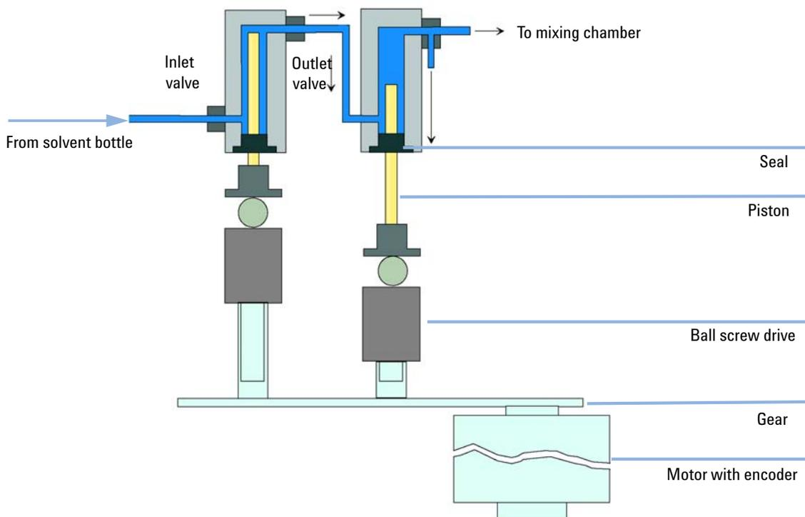
**Figure 3** Principle of Pump Unit
