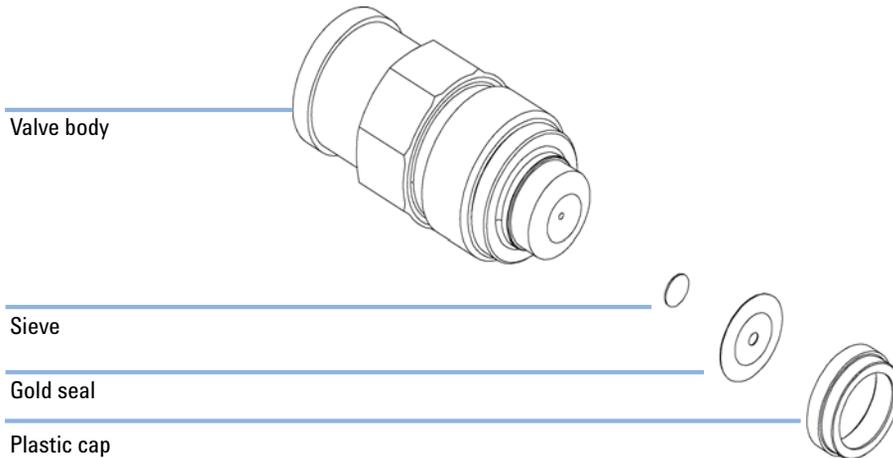
**Figure 18** Outlet Ball Valve Parts
