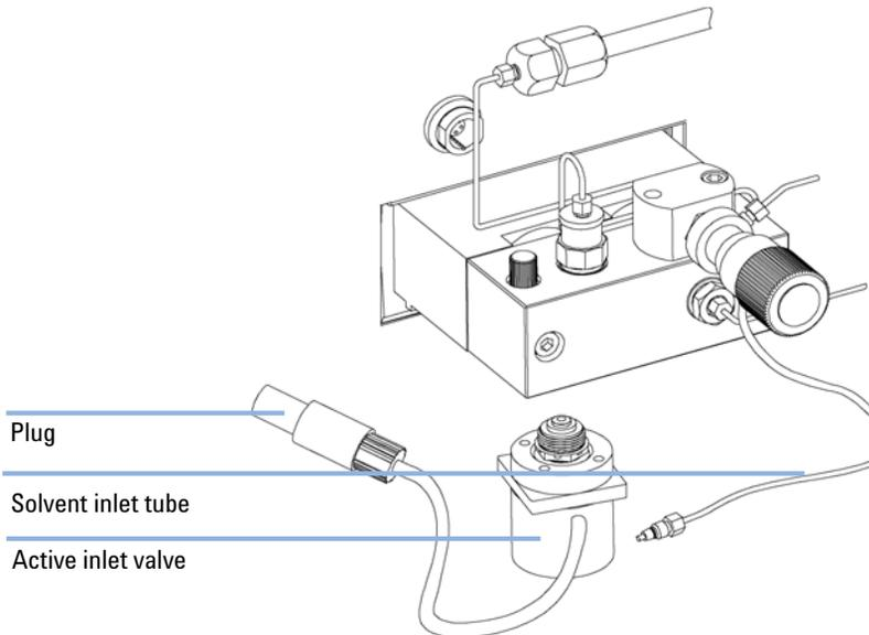
**Figure 16** Exchanging the Active Inlet Valve
