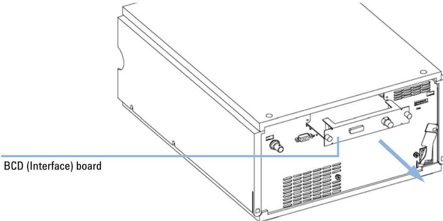
**Figure 27** Exchanging the Interface Board
