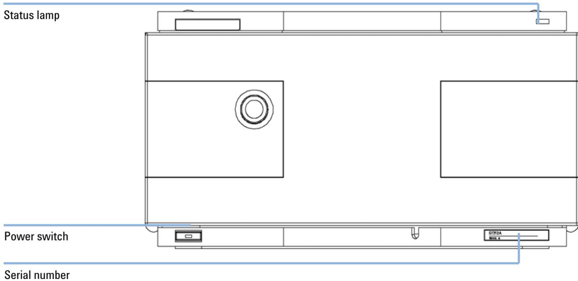
**Figure 7** Front of Binary Pump
