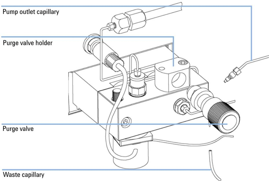
**Figure 21** Exchanging the Purge Valve Frit
