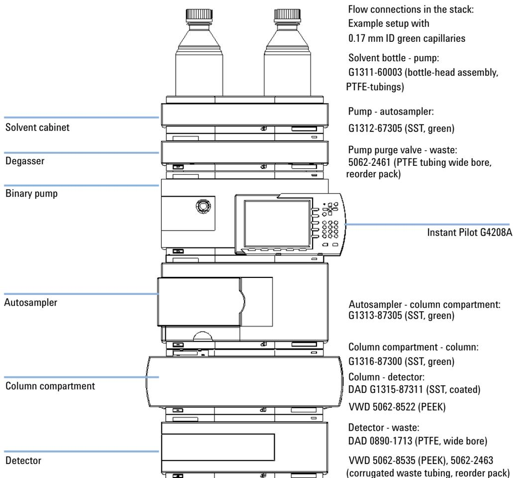
**Figure 5** Recommended Stack Configuration (Front View)
