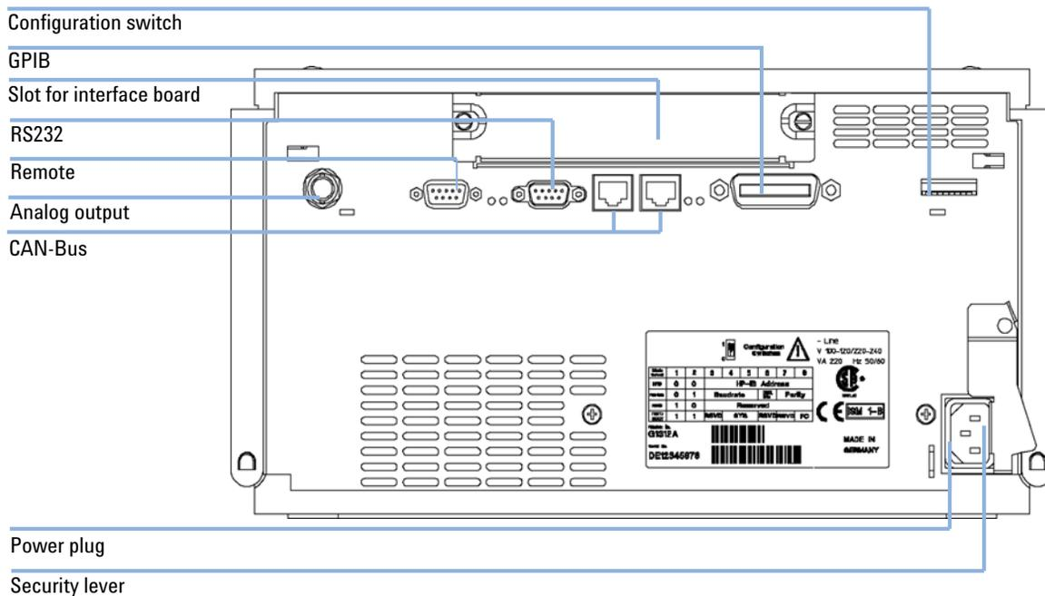
**Figure 8** Rear of Binary Pump
