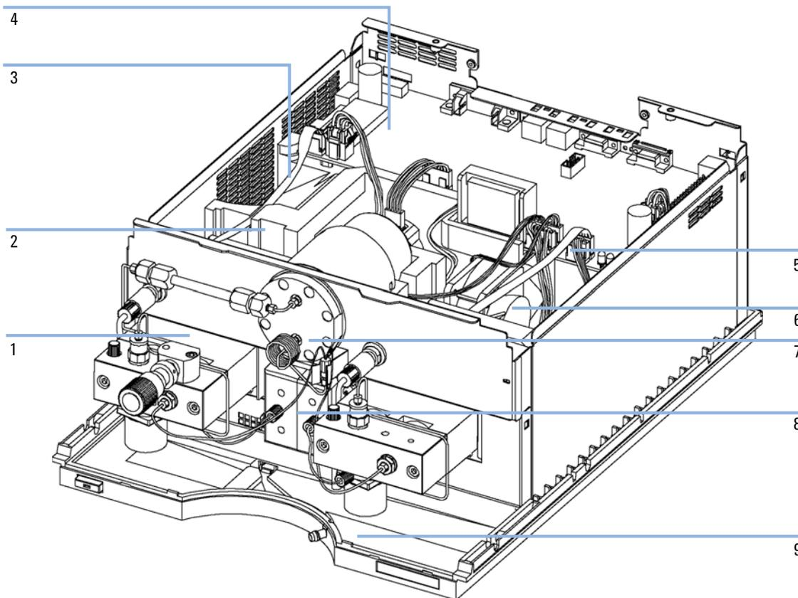
**Figure 28** Overview of Main Assemblies (Front View)
