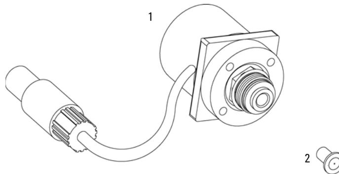
**Figure 34** Active Inlet Valve Assembly
